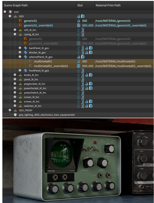
Figure 12: Hierarchical Replacement. The existing glossy substance is replaced with a metal substance on the outer shell by assigning the metal to the same slot name as the glossy, lower in the hierarchy. Copyright © 2022 Animal Logic Pty Ltd. All Rights Reserved.
