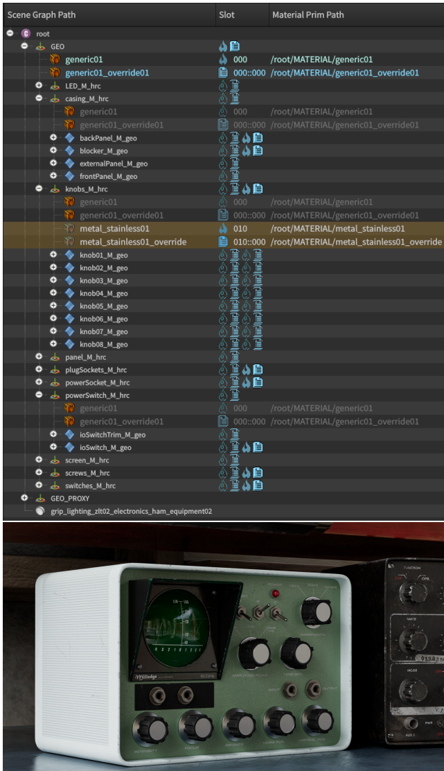
Figure 11: Substance Overrides. A new metal substance (with accompanying override) is assigned to a higher slot lower in the hierarchy, this applies only to the metal elements behind the knobs. Copyright © 2022 Animal Logic Pty Ltd. All Rights Reserved.
